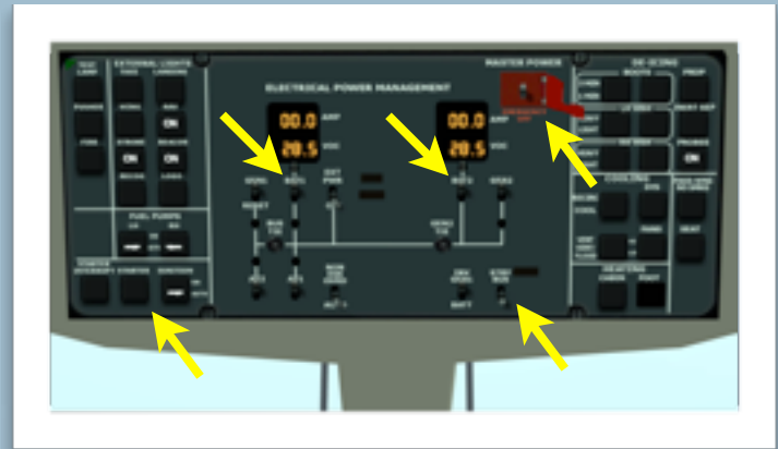
Master Power, Battery, Standby Bus, and Starter switch locations.
