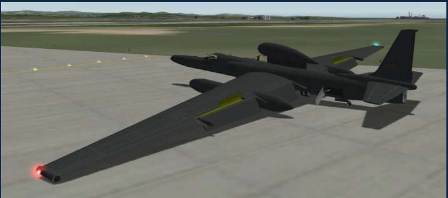
Figure 3. U-2 Flight Control Surfaces Post Landing (before Pogo installation)
